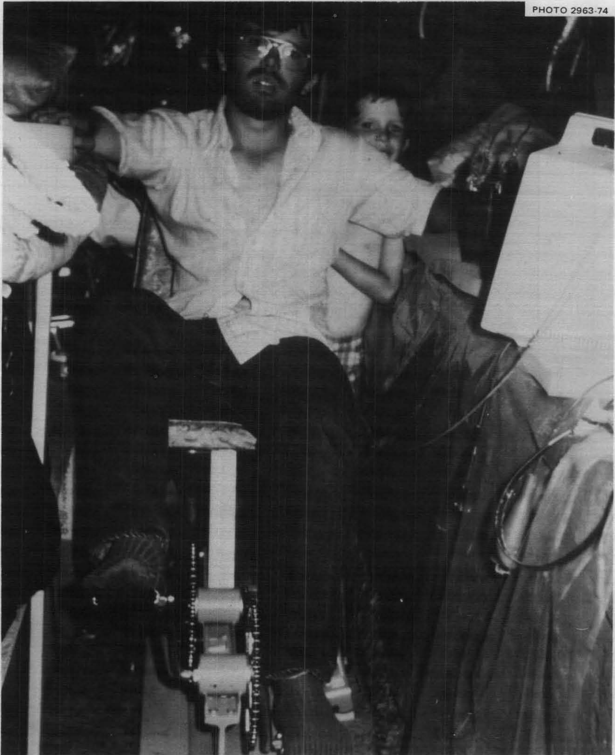
Fig. 4.20. The 18-year-old son getting good exercise by peddling his father's homemade generator to operate their portable TV set. Several years ago the father made this manually powered generator, which uses the sprockets and chains of two bicycles, mounted on a steel frame, to rotate the alternator from a car. The alternator is mounted on a bracket. Only a few minutes were required to remove the alternator and attach it securely to the bracket.
